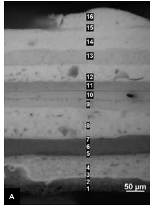
JOSEF FRANK AND OSKAR WLACH, VILLA BEER IN VIENNA-HIETZING, 1930, PAINTS ON METAL, SECTIONS OF SAMPLES; BINDERS: LINSEED OIL OR ALKYD VARNISH; A) FAÇADE, MAIN ENTRANCE, DOOR FRAME METAL, "JAPAN RED", 1: MINIUM PRIMER WITH SOME IRON OXIDE RED, 2: PRIMER: CHALK, ZINC WHITE OR ZINC SICCATIVE / DRIP NOSE, 3: TITANIUM WHITE KRONOS (?), CHALK, 4: TITANIUM WHITE, SILICATES (FINE SAND), 5: LEAD CHROMATE AS BICHROMATE, RED, 6: LEAD CHROMATE AS (5), ORANGE RED. 7 – 16: LATER COATINGS; B) MEZZANINE, SERVICE STAIRS, UPRIGHT, LIGHT YELLOW, 1: MINIUM, IRON OXIDE, CHALK, 2: BARITE, ZINC WHITE YELLOW OCHER (ORIGINAL SURFACE).
